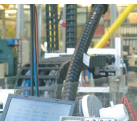
Test a torsione su catene e cavi Torsion test-set for Chainflex®-cables and Triflex® R
