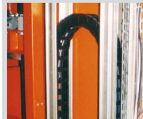
Manipolatore con catena portacavi verticale in piedi e canale di guida in alluminio E-Chain® on the tower of the storage and retrieval unit for high-bay warehouses rolls off from one aluminum guide trough to the opposite one
