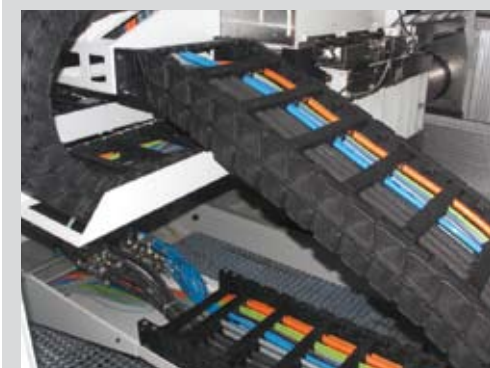
Catena portacavi preassemblata con cavi Chainflex® Pre-harnessed E-Chain® with Chainflex® cables
